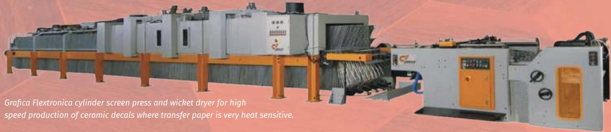
*Grafica Flextronica cylinder screen press and wicket dryer for high speed production of ceramic decals where transfer paper is very heat sensitive.*
