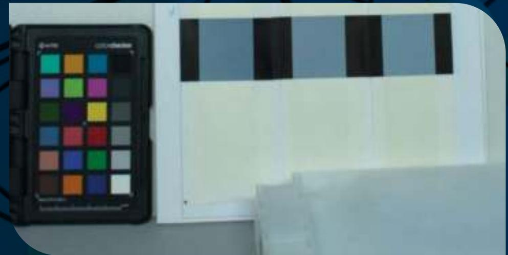
*There are many ISO standards available to help evaluate the printability and durability of a certain substrate. Here a test of the opacity of white ink printed digitally on a dark substrate.*
