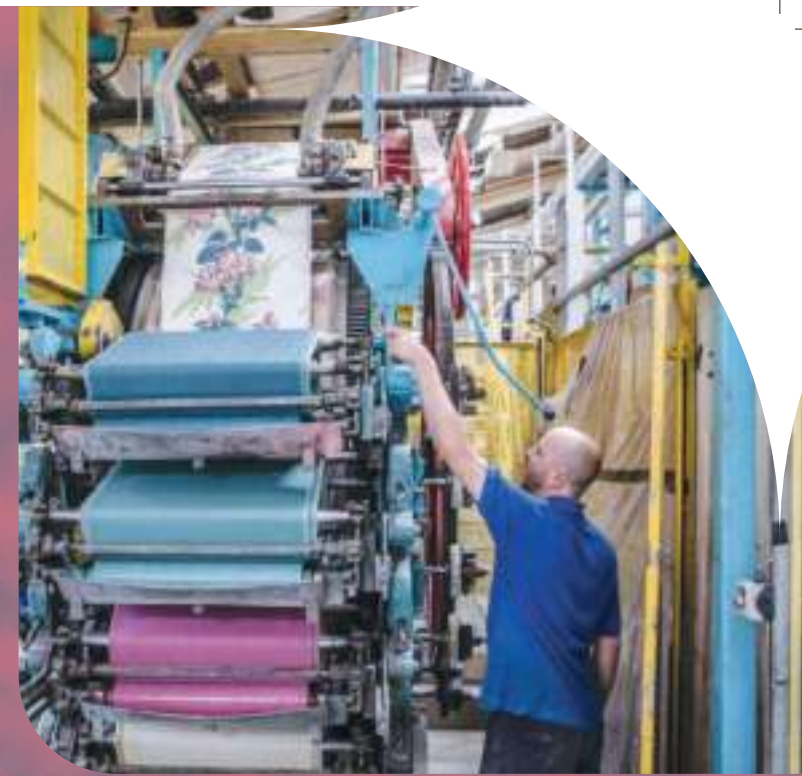
Traditional wallpaper flexo press Image courtesy of Surfaceprint.
