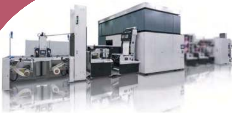
PG Prints offer volume printers the PIKE décor 700 single pass press running at 70 metres per minute.
