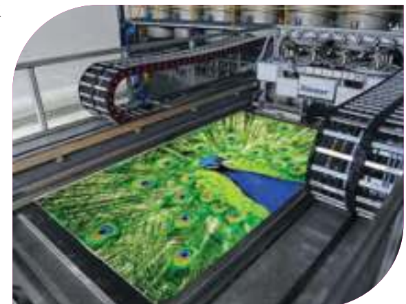
Zimmer multi-pass inkjet for industrial carpet print production.
