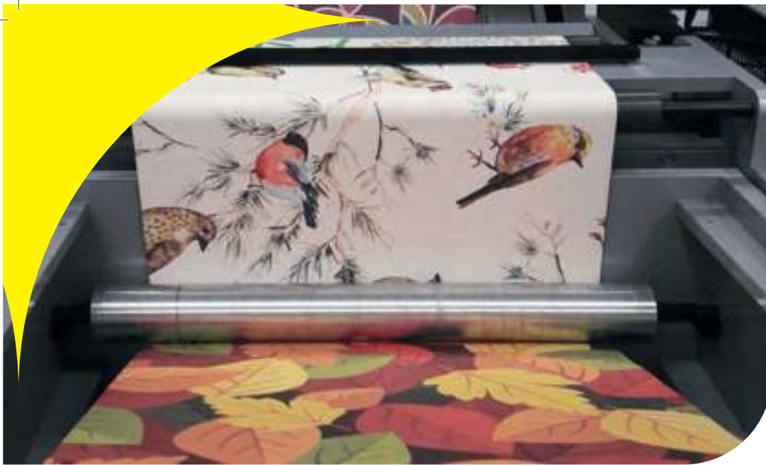
III Single pass inkjet developed with Konica Minolta for high speed mass customization.
