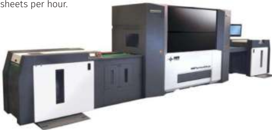
SEI PaperOne 5000 Laser B2 cutter for substrates up to 600 microns thick. It also features a digital creasing matrix option using male female plate. It has a production speed of 2,500 sheets per hour.
