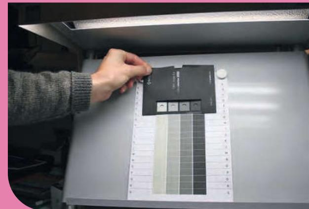
*If OBA is suspected in the printing or proofing paper, the appearance can be determined with the help of the X-Rite ColorChecker PROOF reference.*
